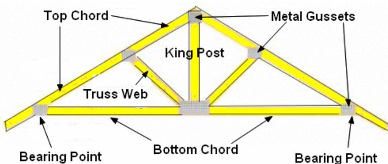
All of the existing federal period buildings in Old Towne originally had gabled roofs made of common roof trusses. The term "gable" refers to the outside wall.
